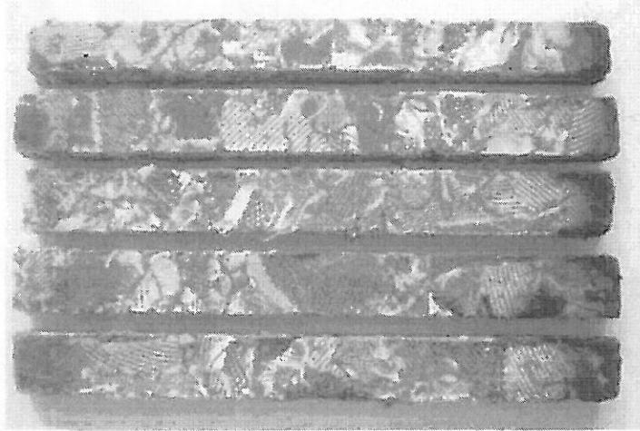
Test Specimens after UL94 Vertical Test
